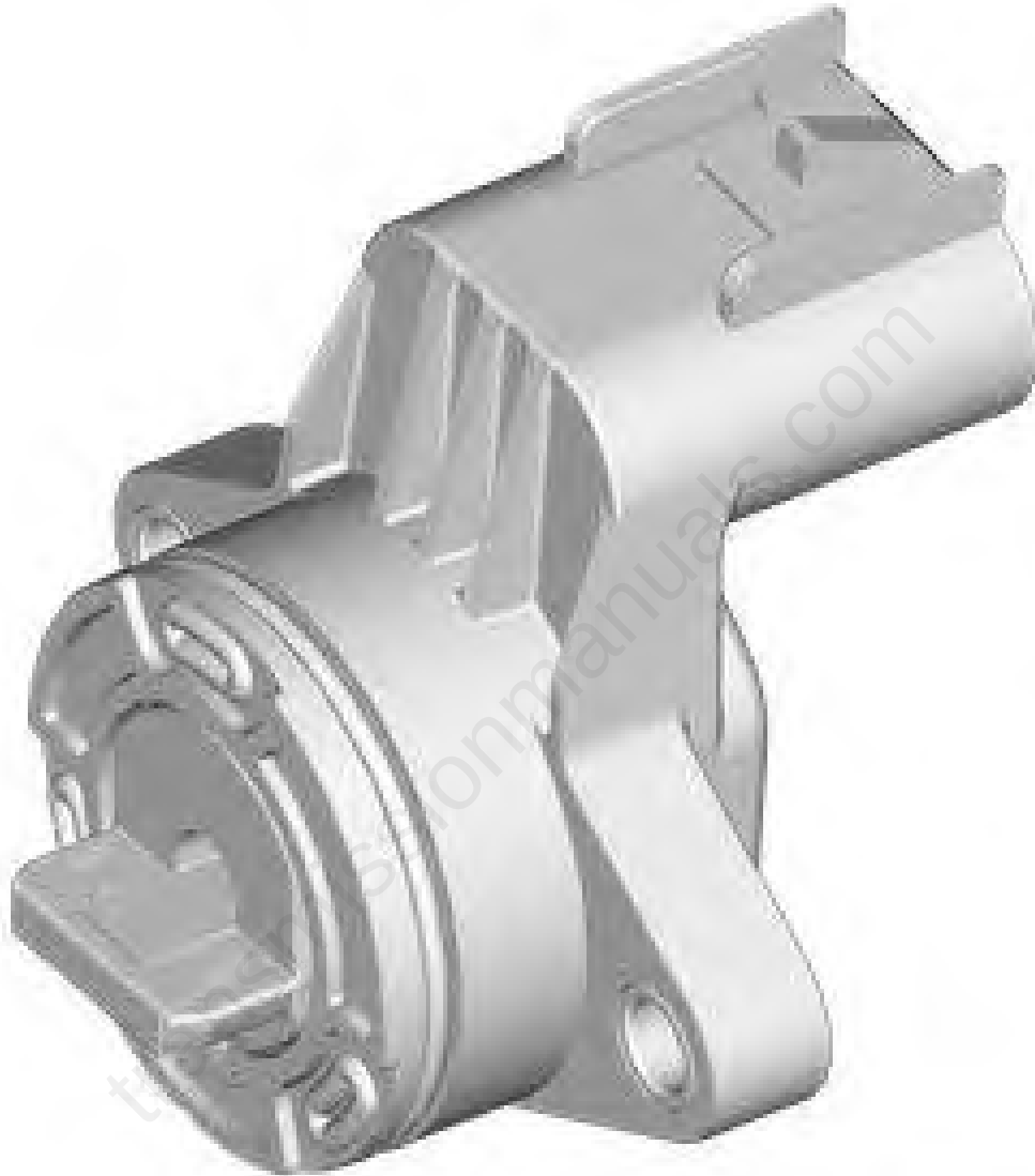
Fig. 90: Transfer Case Actuator Shaft Position Sensor Assembly Courtesy of GENERAL MOTORS COMPANY
